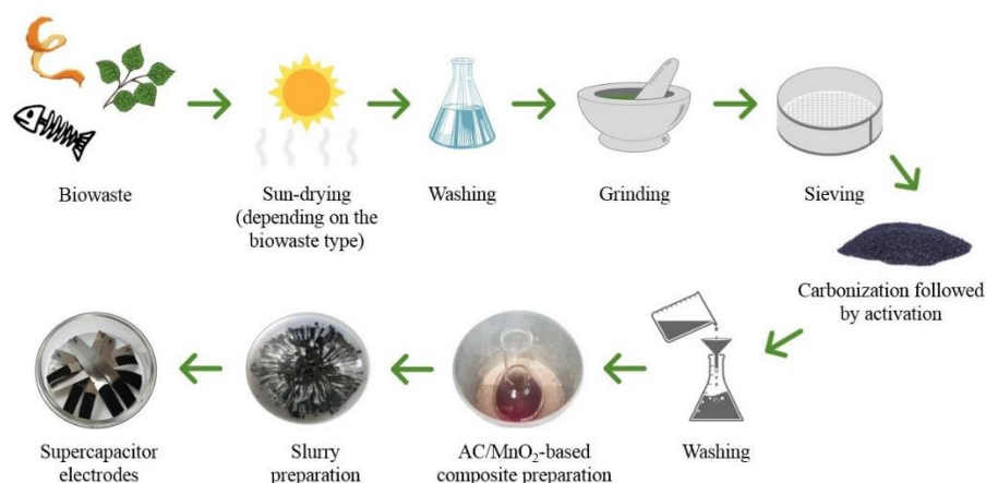
Figure 4. Scheme of preparation of biowaste-derived AC/ \text{MnO}_2 -based composite for supercapacitor electrodes. This figure was created by using the Canva application.
